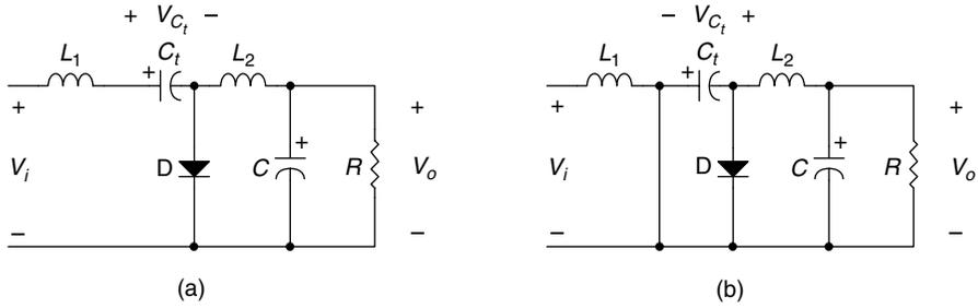
**FIGURE 2.25** Cúk converter switch states: (a) switch open; (b) switch closed. (From Mohan, N., Undeland, T. M., and Robbins, W. P., *Power Electronics: Converters, Applications, and Design*, 2nd ed., John Wiley & Sons, New York, 1995. With permission from John Wiley & Sons.)
