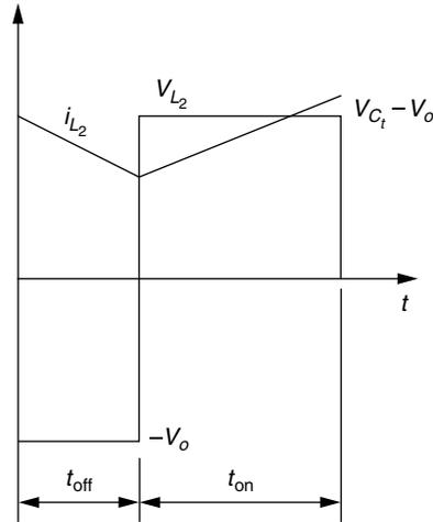
**FIGURE 2.27** Inductor 2, voltage and current waveforms for Cúk converter. (From Mohan, N., Undeland, T. M., and Robbins, W. P., *Power Electronics: Converters, Applications, and Design*, 2nd ed., John Wiley & Sons, New York, 1995. With permission from John Wiley & Sons.)
