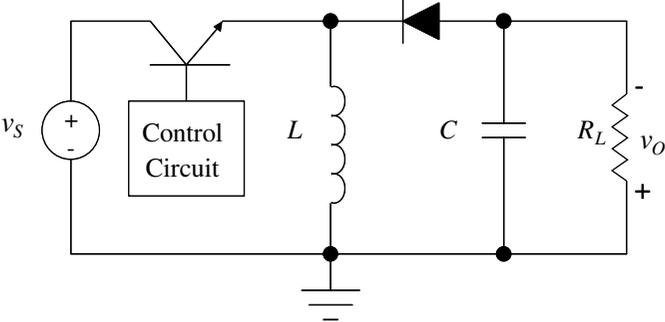
FIGURE 2.28 Buck–boost converter.
