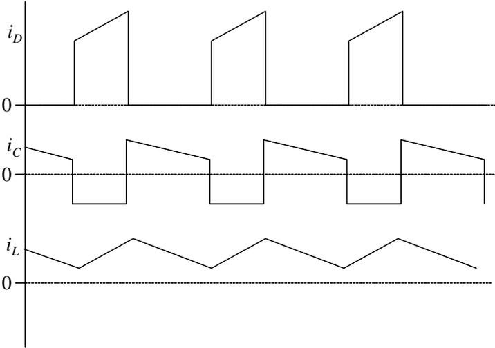
FIGURE 2.29 Typical current waveforms in a buck–boost converter.
