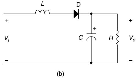
**FIGURE 2.21** Basic boost converter switch states: (a) switch closed; (b) switch open. (From Mohan, N., Undeland, T. M., and Robbins, W. P., *Power Electronics: Converters, Applications, and Design*, 2nd ed., John Wiley & Sons, New York, 1995. With permission from John Wiley & Sons.)
