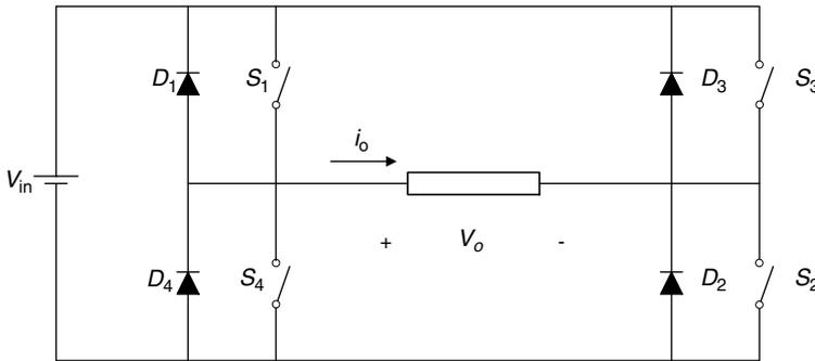
FIGURE 2.11 A full-bridge four-quadrant chopper.
