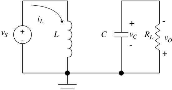
FIGURE 2.30 Topology 1 for the buck–boost converter.
