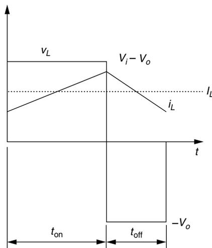
**FIGURE 2.18** Inductor voltage and current for continuous mode of buck converter. (From Mohan, N., Undeland, T. M., and Robbins, W. P., *Power Electronics: Converters, Applications, and Design*, 2nd ed., John Wiley & Sons, New York, 1995. With permission from John Wiley & Sons.)
