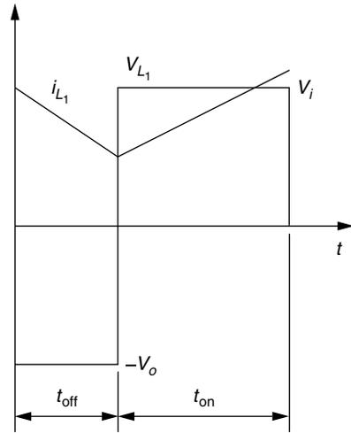
**FIGURE 2.26** Inductor 1, voltage and current waveforms for Cúk converter. (From Mohan, N., Undeland, T. M., and Robbins, W. P., *Power Electronics: Converters, Applications, and Design*, 2nd ed., John Wiley & Sons, New York, 1995. With permission from John Wiley & Sons.)
