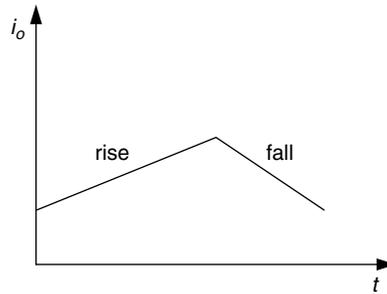
**FIGURE 2.15** Rise and fall of load current in buck converter.
