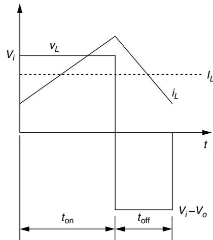
**FIGURE 2.22** Inductor voltage and current waveforms for continuous mode of boost converter. (From Mohan, N., Undeland, T. M., and Robbins, W. P., *Power Electronics: Converters, Applications, and Design*, 2nd ed., John Wiley & Sons, New York, 1995. With permission from John Wiley & Sons.)
