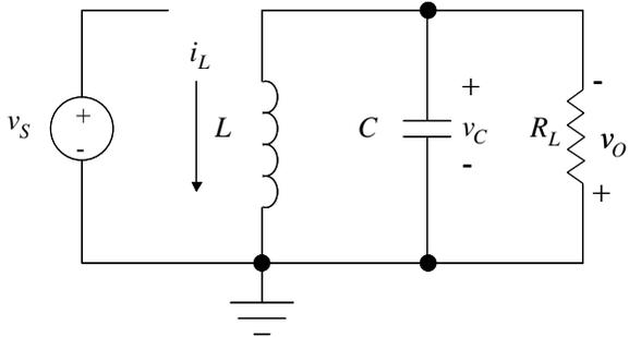
FIGURE 2.31 Topology 2 for the buck–boost converter.
