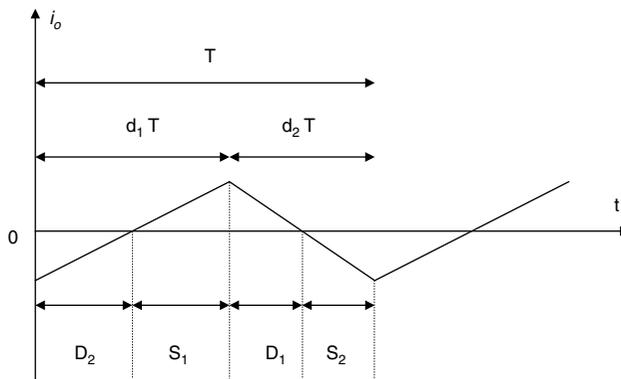
FIGURE 2.9 Output current of a two-quadrant chopper.
