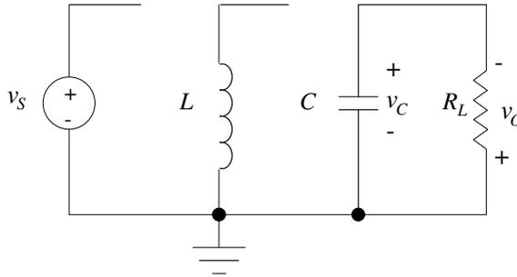
FIGURE 2.37 Topology 3 for the buck–boost converter (discontinuous inductor current).
