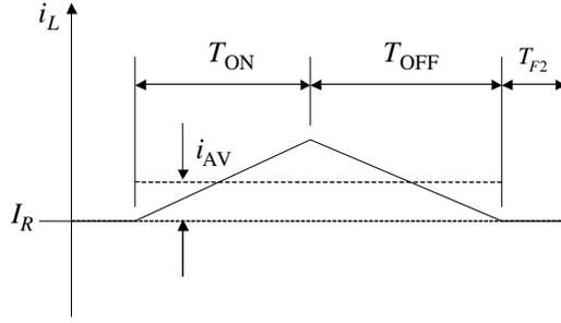
FIGURE 2.38 General form of discontinuous inductor current.
