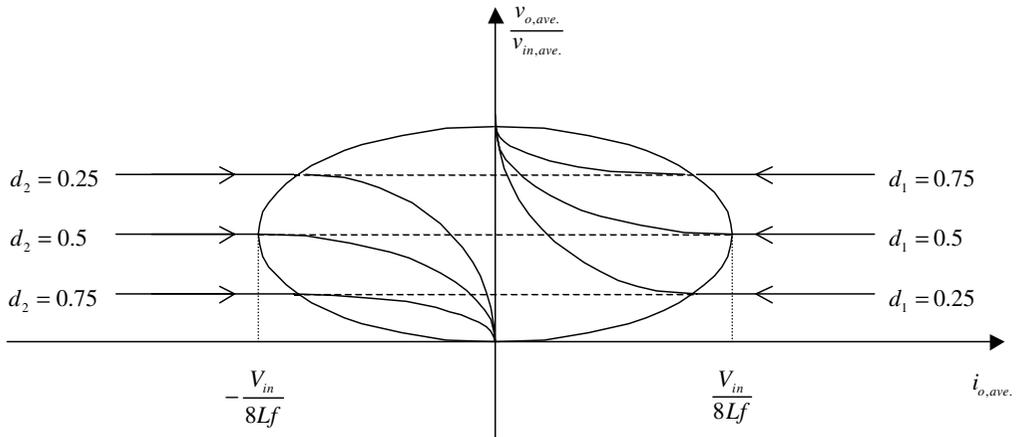
FIGURE 2.10  $(v_{o,ave.}/v_{in,ave.}) - i_{o,ave.}$  characteristic of a two-quadrant converter.
