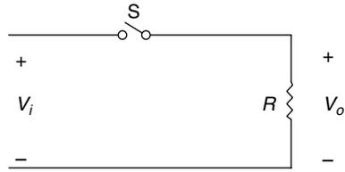
FIGURE 2.1 Basic DC-DC converter.
