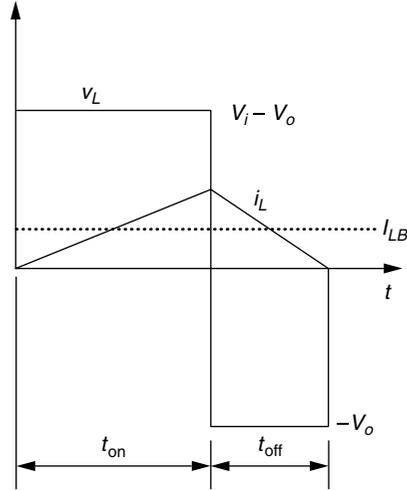
**FIGURE 2.19** Inductor current at boundary point for discontinuous mode of buck converter. (From Mohan, N., Undeland, T. M., and Robbins, W. P., *Power Electronics: Converters, Applications, and Design*, 2nd ed., John Wiley & Sons, New York, 1995. With permission from John Wiley & Sons.)
