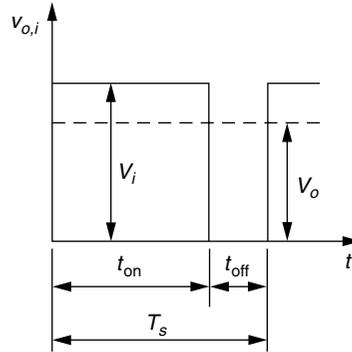
FIGURE 2.2 DC-DC converter voltage waveforms. (From Mohan, N., Undeland, T. M., and Robbins, W. P., *Power Electronics: Converters, Applications, and Design*, 2nd ed., John Wiley & Sons, New York, 1995. With permission from John Wiley & Sons.)
