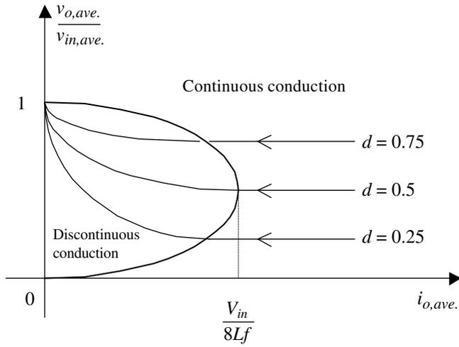
FIGURE 2.5  $(v_{o,ave.}/v_{in,ave.}) - i_{o,ave.}$  characteristic of a step-down converter.
