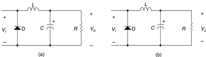
**FIGURE 2.17** Buck converter switch states: (a) switch in position 1; (b) switch in position 2. (From Mohan, N., Undeland, T. M., and Robbins, W. P., *Power Electronics: Converters, Applications, and Design*, 2nd ed., John Wiley & Sons, New York, 1995. With permission from John Wiley & Sons.)
