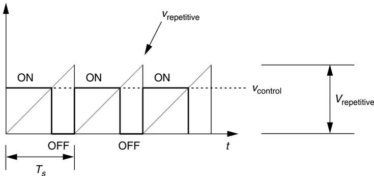
FIGURE 2.3 Pulsewidth modulation concept. (From Mohan, N., Undeland, T. M., and Robbins, W. P., *Power Electronics: Converters, Applications, and Design*, 2nd ed., John Wiley & Sons, New York, 1995. With permission from John Wiley & Sons.)
