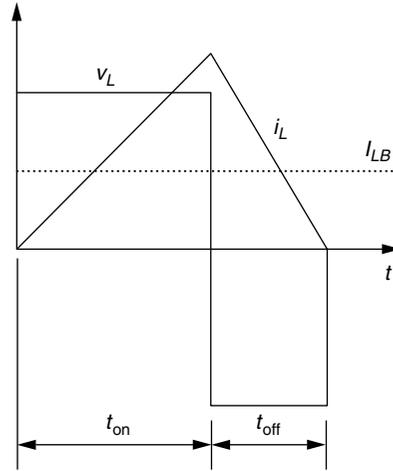
**FIGURE 2.23** Inductor current at boundary point for discontinuous mode of boost converter. (From Mohan, N., Undeland, T. M., and Robbins, W. P., *Power Electronics: Converters, Applications, and Design*, 2nd ed., John Wiley & Sons, New York, 1995. With permission from John Wiley & Sons.)
