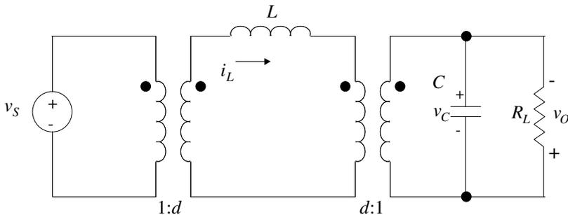
FIGURE 2.34 Average circuit model of the buck–boost converter.
