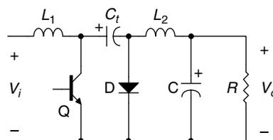
**FIGURE 2.24** Nonisolated Cúk converter. (From Mohan, N., Undeland, T. M., and Robbins, W. P., *Power Electronics: Converters, Applications, and Design*, 2nd ed., John Wiley & Sons, New York, 1995. With permission from John Wiley & Sons.)
