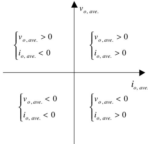
FIGURE 2.12 Four-quadrant operation of a full-bridge chopper.
