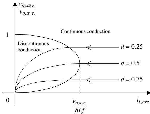
FIGURE 2.7  $(v_{in,ave.}/v_{o,ave.}) - i_{L,ave.}$  characteristic of a step-down converter.
